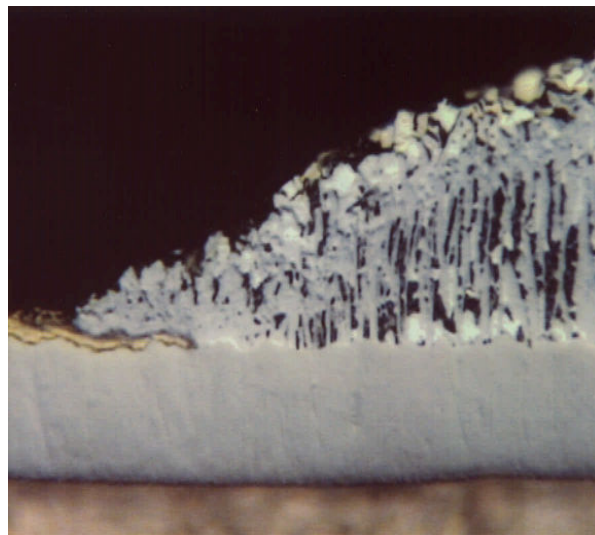
Figure 8-Concentrated Au-Sn IMC at leading edge of Solder as it reacts with Au deposit.
