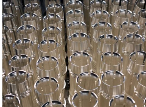
Figure 3: Bright Silver Plated Machined C147 Copper Finger Contacts
