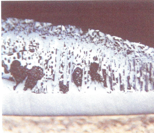
Figure 7- Concentration of Au-Sn and Ni-Sn IMC at reaction interface with Solder.
