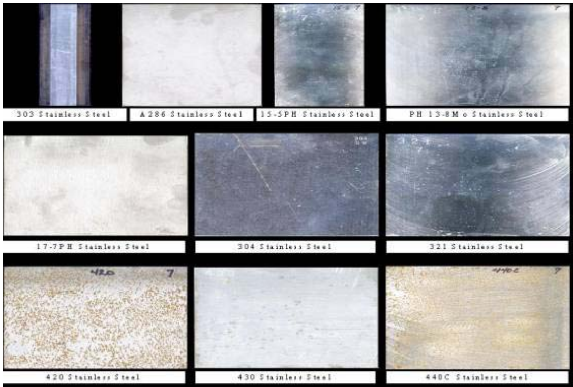
Figure 1 – As-Received Stainless Steel Test Specimens Subjected to 2 Hour Salt Spray. Test Specimens Did Not Receive a Passivation Treatment.
