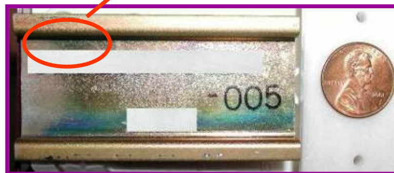
Zinc Whiskers Growing from Zinc-Plated Yellow Chromate Steel Bus Rail
