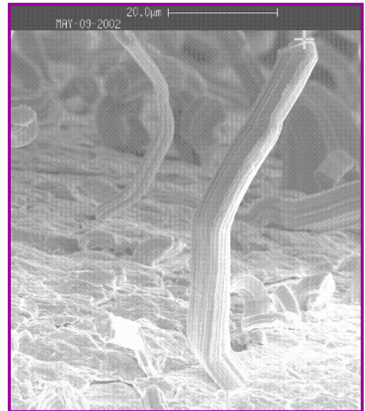
Tin Whiskers on Tin-Plated Ceramic Chip Capacitor
