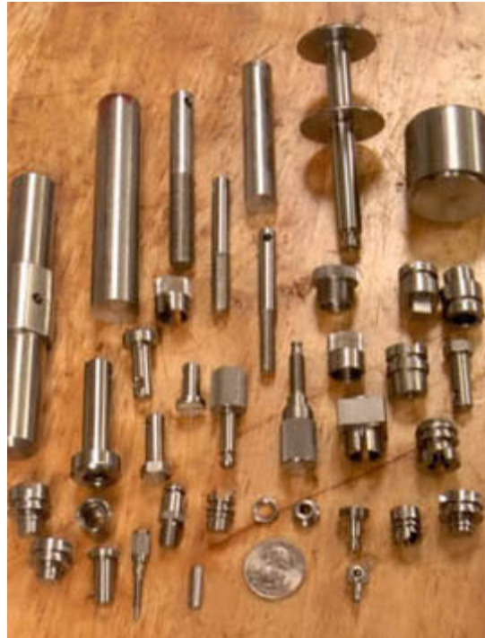
Passivation is designed to maximize the inherent corrosion resistance of stainless steel parts after machining.
