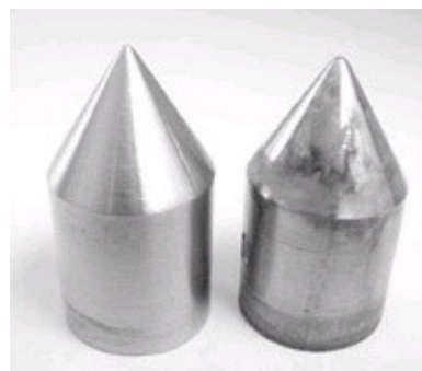
Fig. 3 - Test cone on left shows a bright finish with improved resistance of free-machining stainless
